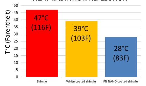
REGULAR SURFACE 47°C (116F) WHITE PAINT (WHITE ROOF SYSTEM) 39°C (102F) FN NANO  $TiO_2$  COATING 28°C (83F)
